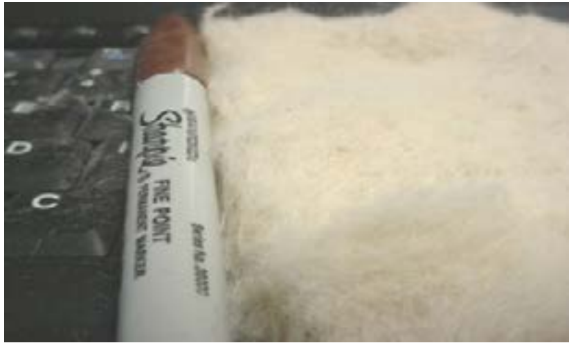
16-Hour Dust Accumulation (Figure 7)
