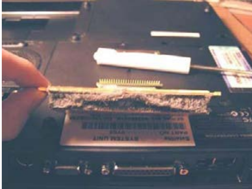
Laptop Fibrous Dust Clogging (Figure 2)
