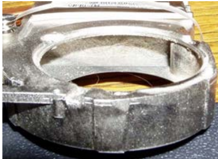
Clogged Heat Sink Fins (Figure 1)
