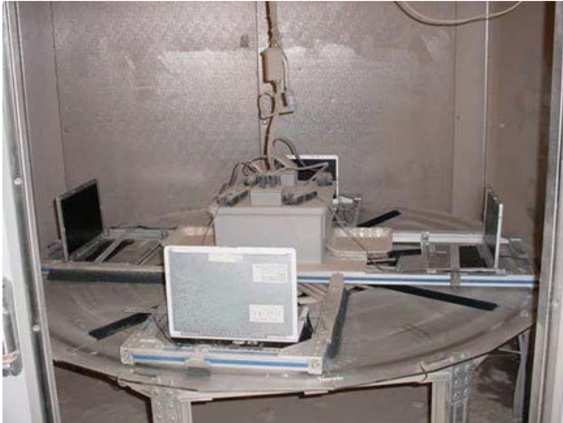
Dust Test Chamber Accommodates Active/Passive Testing. (Figure 11)
